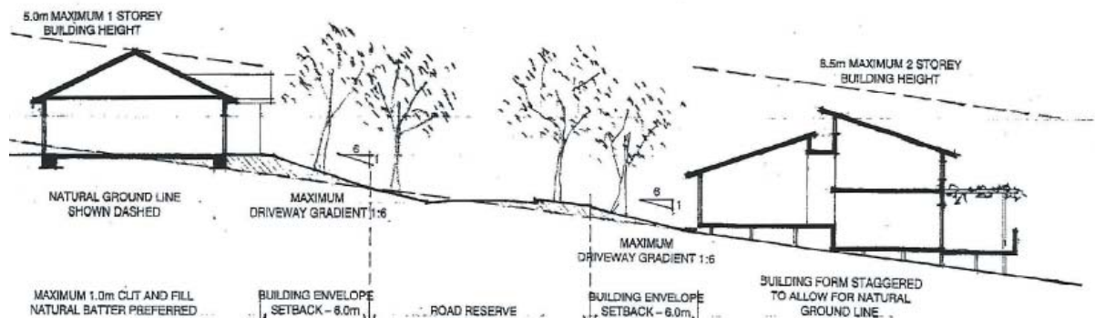
Section Demonstrating Excavation and Fill (MR 6)
